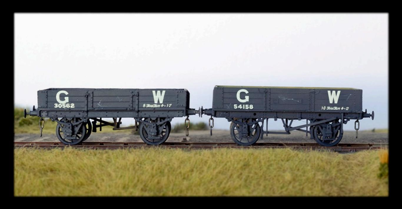
A 3 plank wagon built from a David Geen kit and a four-plank wagon. Cooper Craft sides and ends with a Morgan underframe and other parts as mentioned in the main part of the text. Both are modelled as wagons in the 25" livery period. Neither wagon can fit 25" lettering and the 3 plank used something around 18" and the 4 plank used 20" (approx.) The closest available is 16" lettering so that has to do and I used this in both cases. Neither wagon has been weathered yet, that is the next project.
