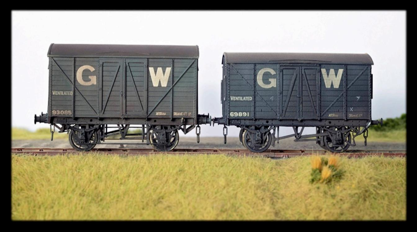
The same V16 van with a V5 van. The V5 is built from the Coopercraft kit and was built with Bill Bedford Irons and Masokits brake gear. The brakegear in the Coopercraft kits is lacking and the kits really do benefit from better brake gear. I have fitted ventilated ends using a set from some spare ends that CC supplied at one point. I have not seen a photo of a V5 so fitted and I have some concerns about whether it actually existed. The next V5 will be built as a non-ventilated wagon.
